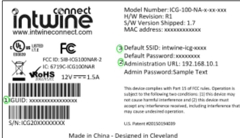
A variant of the above pictured label ships on every production 4GR with both standard information and information that is specific to each individual Gateway. The label is full of pertinent information including the 4GR's FCC ID, UL number, MAC address, serial numbers, etc. The three most important pieces of information for configuring the 4GR are labeled above and described below:
