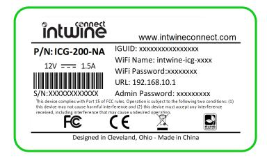
A variant of the above pictured label ships on every production ICG-200 with both standard information and information that is specific to each individual Gateway. The label is full of pertinent information including the router's FCC ID, UL number, MAC address, serial numbers, etc. The three most important pieces of information for configuring the ICG-200 are labeled above and described below:
